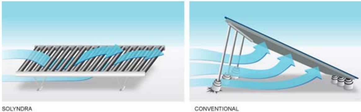
Figure 18 - Wind design for Solyndra and a conventional system.
